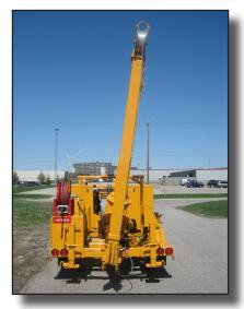
Optional fully hydraulic controlled telescopic boom with vertical lift allows easy maneuvering of boom into manholes with varying approach angles.
