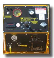
Permanently engraved operator's panel with user friendly controls. Infinitely variable line speed and tension control with automatic overpull protection.
