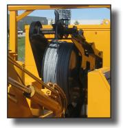
Storage reel with 701 m (2300 ft.) of 11 mm (7/16") diameter rotation resistant wire pulling rope. Automatic levelwind included with unit.
