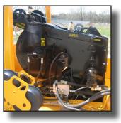
Unique hydraulic bullwheel drive system provides constant pulling force and speed throughout the entire pull; includes payout on demand feature allow direct blowing of pulling rope into duct.
